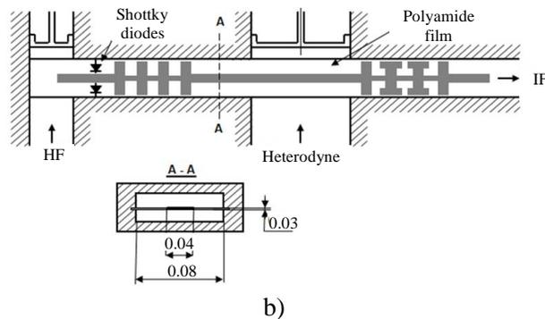
**FIG. 4:** Block circuit (a) and design (b) diagrams of the converter
