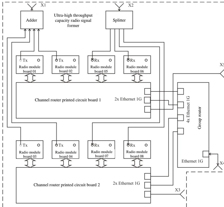
**FIG. 2:** Block circuit diagram of the Gigabit modem
