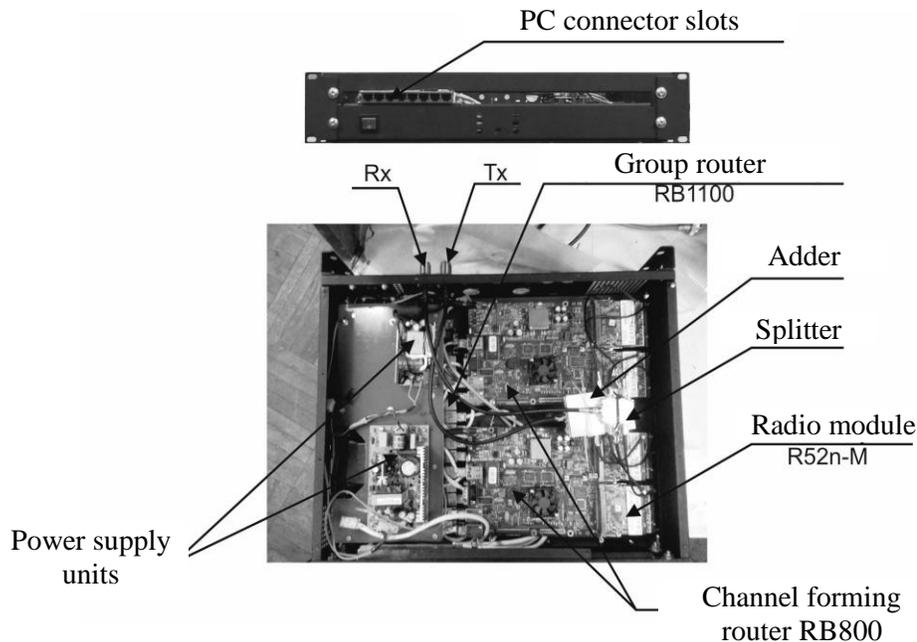
**FIG. 3:** Photographic image of the G Gigabit modem laboratory sample
