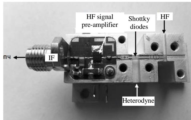
**FIG. 5:** Design of the frequency converter
