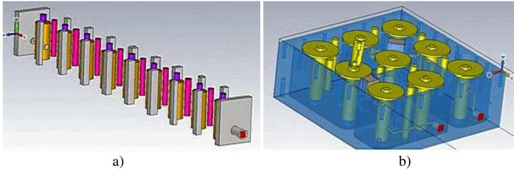
**FIG. 2:** Simplified 3D filter models: a) 1920-1980 MHz and 2510-2570 MHz; b) 820-843 MHz and 890-915 MHz
