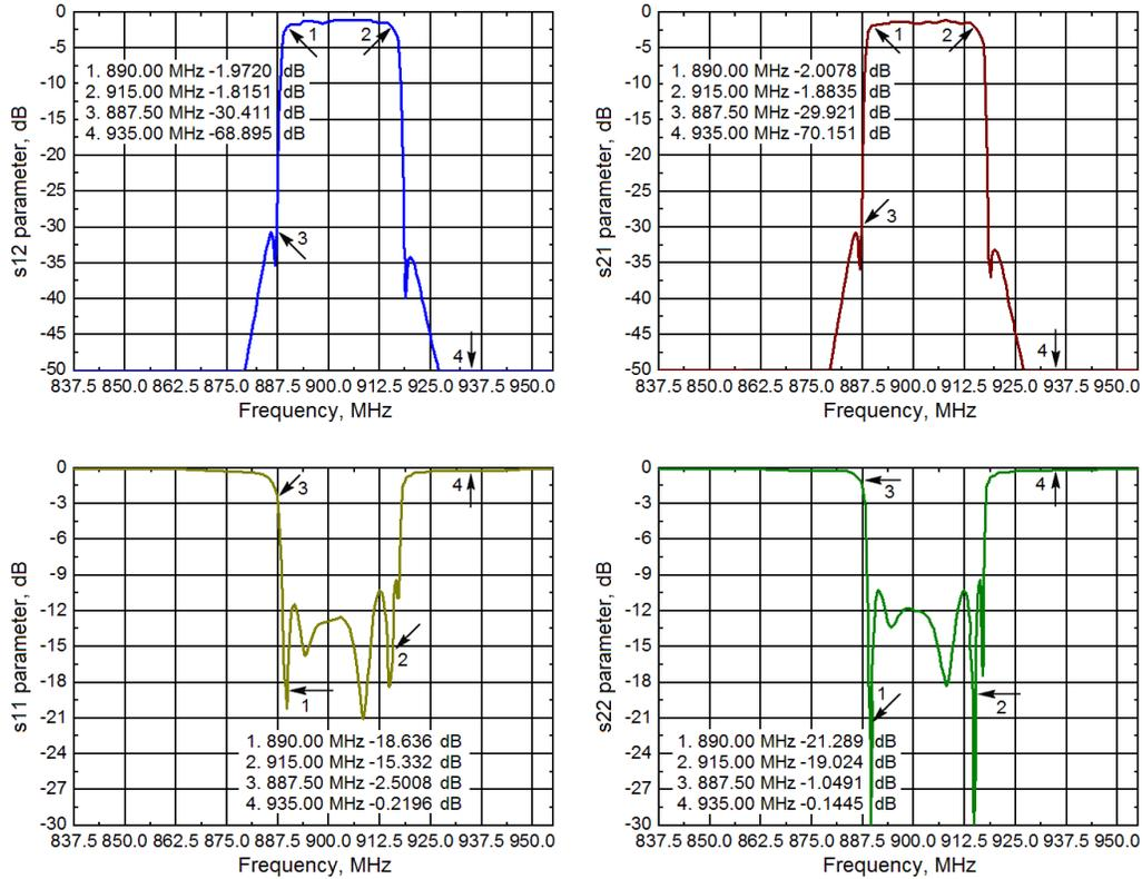
**FIG. 5:** Measured amplitude-frequency characteristics and frequency characteristics of the reflection coefficient for “BF -890-2-30” band-pass filter
