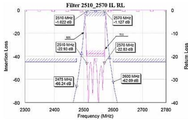
**FIG. 3:** Simulated amplitude-frequency characteristic and frequency characteristic of the reflection coefficient of the 2510-2570 MHz filter
