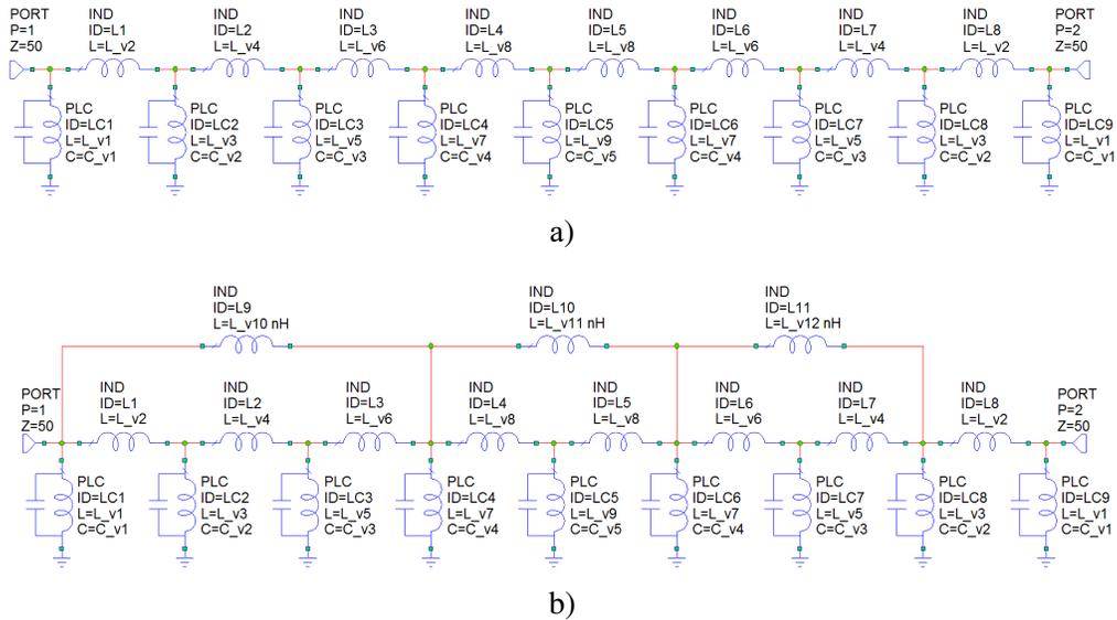
**FIG. 1:** Electric circuits of low-frequency prototypes: a) 1920-1980 MHz and 2510-2570 MHz filters; b) 820-843 MHz and 890-915 MHz cross-links filters
