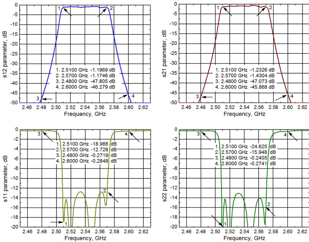
**FIG. 4:** Measured amplitude-frequency characteristics and frequency characteristics of the reflection coefficient for “BF -2510-2-40” band-pass filter
