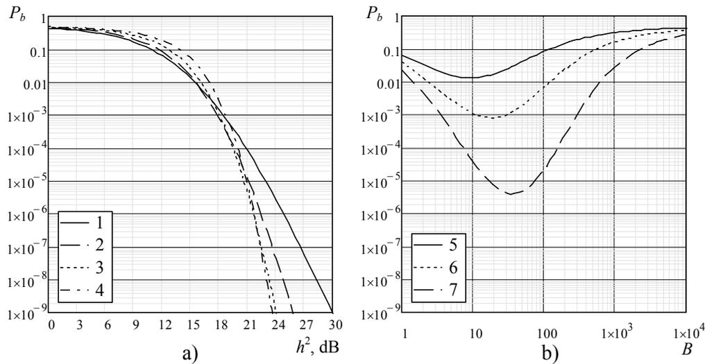
**FIG. 3:** Dependence of  $P_b = P_b(h^2)$  at the fixed bandwidth-delay product  $B$  (1 -  $B=8$  ; 2 -  $B=16$  ; 3 -  $B=32$  ; 4 -  $B=64$  ) (a) and dependence of  $P_b = P_b(B)$  at the fixed  $h^2$  (5 -  $h^2 = 15.051$  dB, 6 -  $h^2 = 18.062$  dB, 7 -  $h^2 = 21.072$  dB) (b) for the communication using ANSK
