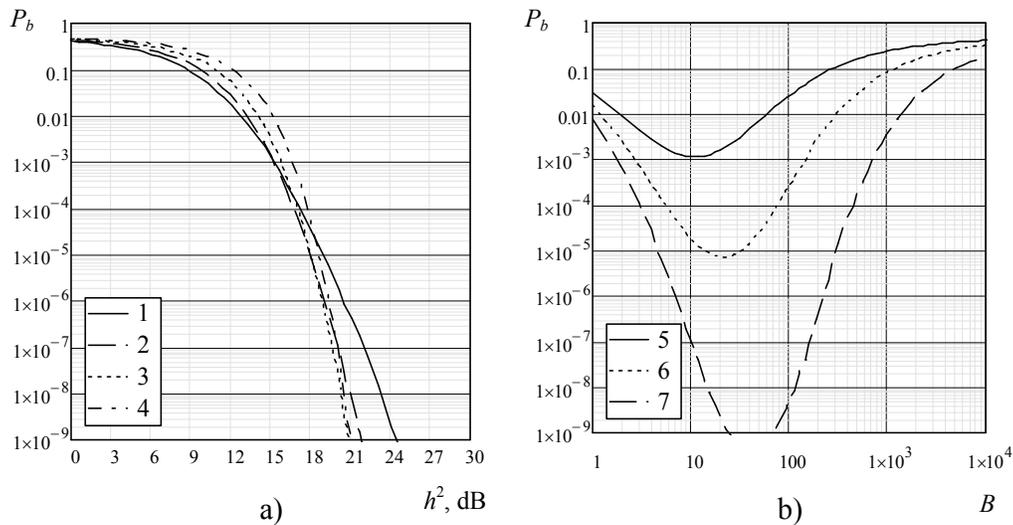
**FIG. 5:** Dependence of  $P_b = P_b(h^2)$  at the fixed bandwidth-delay product  $B$  (1 -  $B=8$ ; 2 -  $B=16$ ; 3 -  $B=32$ ; 4 -  $B=64$ ) (a) and dependence of  $P_b = P_b(B)$  at the fixed  $h^2$  (5 -  $h^2 = 15.051$  dB, 6 -  $h^2 = 18.062$  dB, 7 -  $h^2 = 21.072$  dB) (b) for the communication using FNSK
