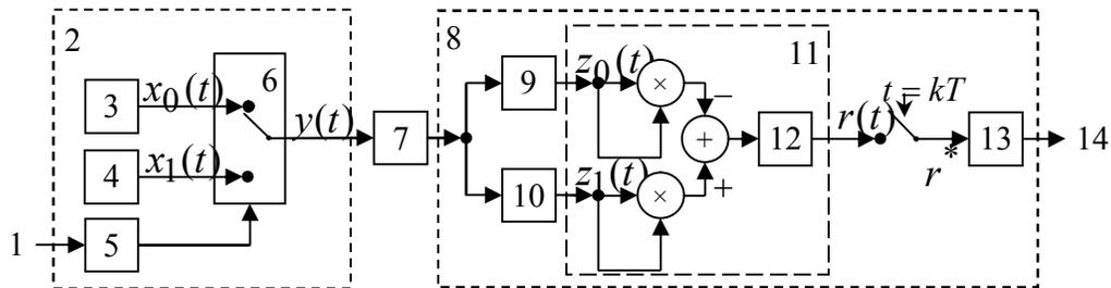
**FIG. 4:** Block diagram of the communication using FNSK: 1 – transmitted bit; 2 – transmitter; 3 – NSG-0; 4 – NSG-1; 5 – encoder; 6 – switch; 7 – channel; 8 – receiver; 9, 10 – bandpass filters; 11 – demodulator; 12 – integrating unit; 13 – detector; 14 – received bit
