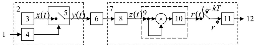
**FIG. 1:** Block diagram of the communication using ANSK: 1 – transmitted bit; 2 – transmitter; 3 – NSG; 4 – encoder; 5 – switch; 6 – channel; 7 – receiver; 8 – bandpass filter; 9 – demodulator; 10 – integrating unit; 11 – detector; 12 – received bit
