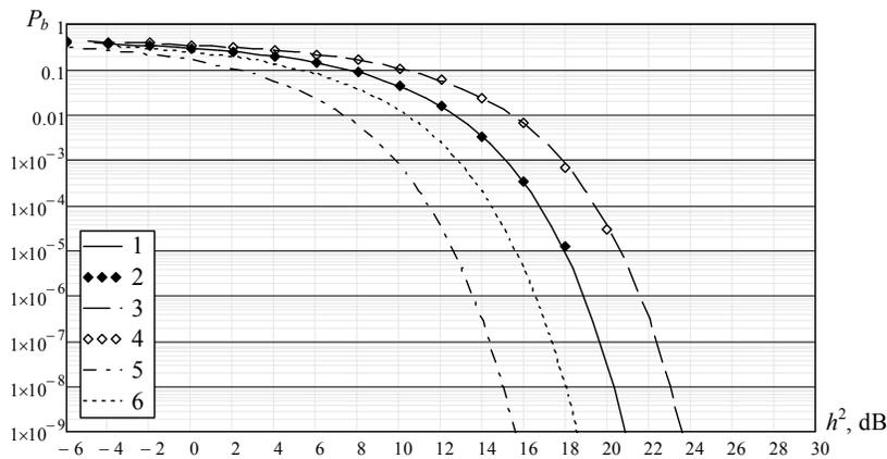
**FIG. 6:** Dependences of  $P_b = P_b(h^2)$  for FNSK (1 - theory, 2 - experiment) and ANSK (3 - theory, 4 - experiment) at optimal parameters. For the purpose of comparison the curves for the frequency (5) and the amplitude (6) noise shift-keying of the deterministic signal are provided
