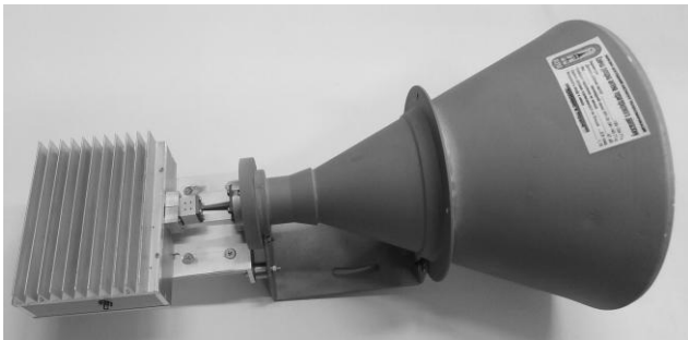
Fig. 10. The view of developed transmitting (receiving) tract of THz wireless system
