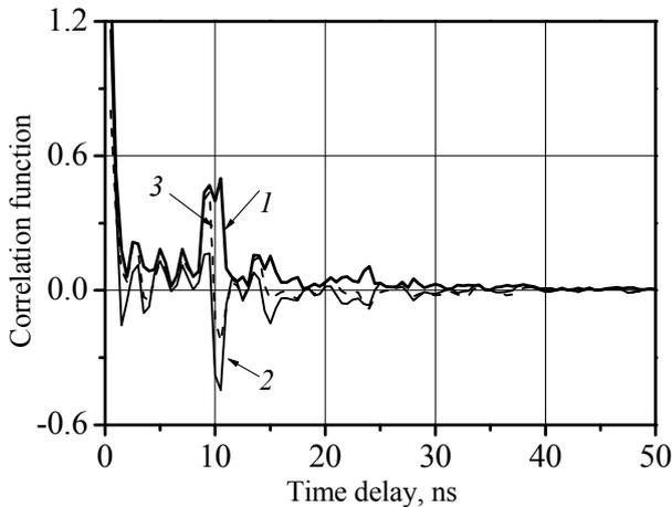
Fig. 3. Complex correlation function of received ultra-wideband noise signal at transmission of bit “1”: (1) envelope; (2) sinusoidal and (3) cosine quadrature components.
