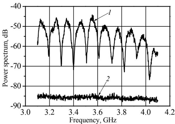
Fig. 2. Power spectrums of received ultra-wideband noise signal (1) with code spectrum modulation and receiver fluctuation noise (2).
