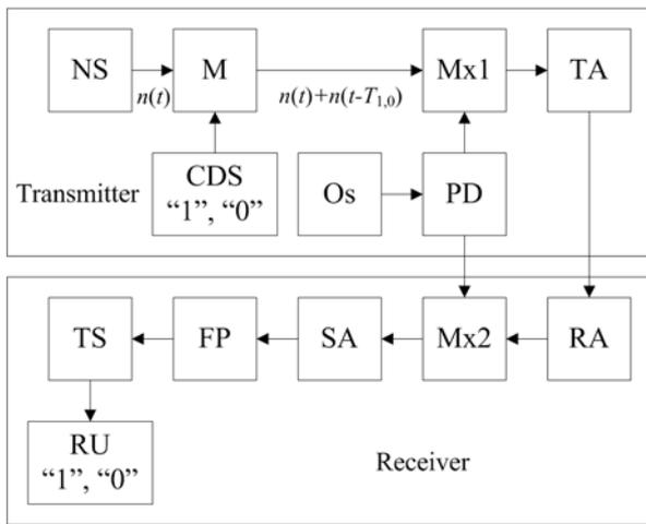
Fig. 1. Block diagram of the transmitter with code spectral modulation and the receiver with double spectral processing.
